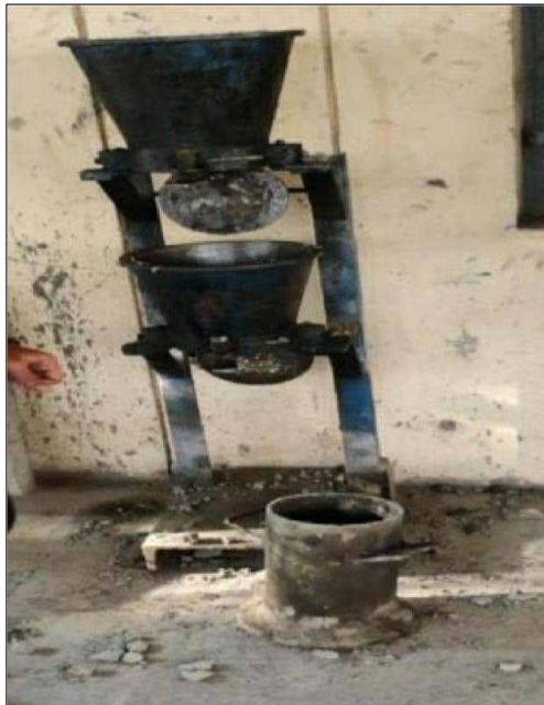
Fig 4: Compaction Factor Test
