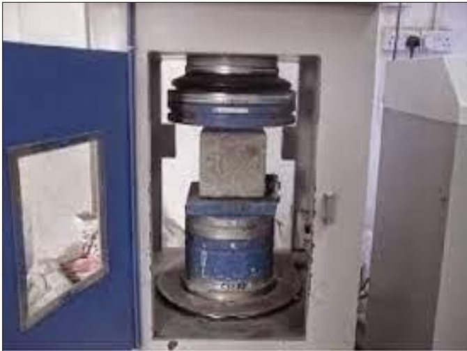
Fig 5: Compressive testing specimen size: cubes (15cm X 15cm 15cm)
